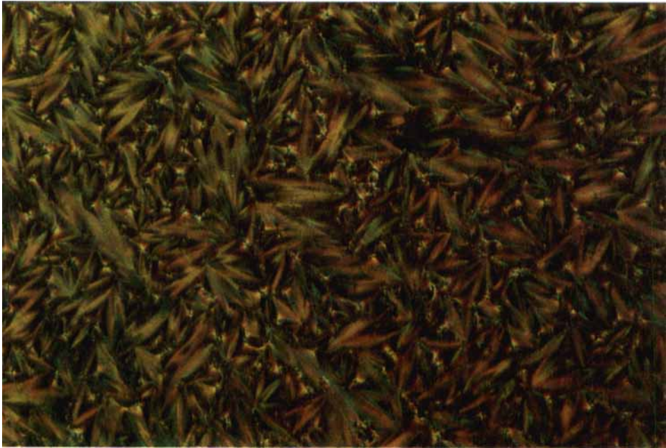
Figure 4. Optical micrograph showing the focal conic defect texture of the smectic C* phase in the complex III at 108°C (cooling cycle), \times 200 .
