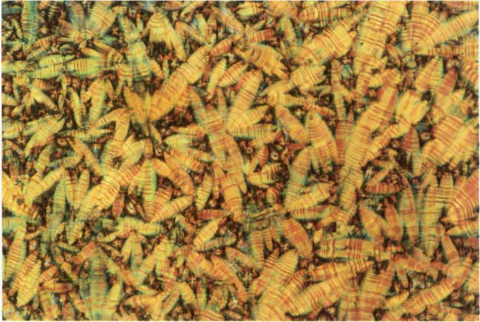
Figure 2. Optical micrograph showing the focal conic defect texture of the smectic C* phase in compound HL 3 at 66°C (cooling cycle), \times 200 .
